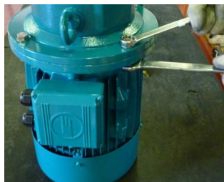
Fig. 29 For pumps with B5 and B14 motor shape, separate the baseplate, position the pump vertically and unscrew the motor locking screws + nuts.
