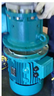
Fig. 30 Separate the pump from the electric motor. Use suitable lifting equipment and pay attention to the attraction of the outer magnet caused by the inner magnet.
