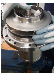
Fig. 36 Unscrew and remove: the impeller nut (922), the washer (931) and the impeller (230).
