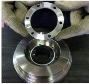
Fig. 47 For the "1st bracket" pumps: extract the locking flange (935) from the bushing support (350).
