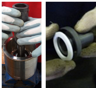
Fig. 41 Extract the following from the impeller shaft (211): the bearing sleeve (529), the rear slewing bearing (510) and then the compensation ring (504).
