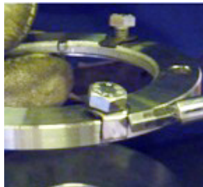
Fig. 53 For the "1st bracket" pumps: insert the hex head screws (901) and their safety washers (931) into the holes of the locking flange (935) and bend the washers over the outer edge of the flange (935).
