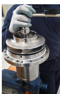
Fig. 36 Unscrew and remove: the impeller nut (922), the washer (931) and the impeller (230).
