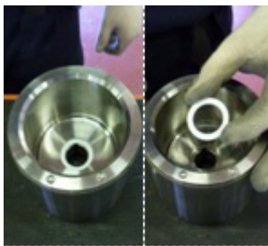
Fig. 50 Slide the bearing sleeve gasket (855) out of the inner magnet (411).
