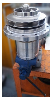
Fig. 35 Tighten the equipment (if available) in a bench vice and place the assembled bracket on top.
