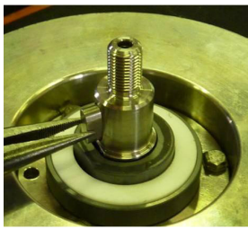
Fig. 38 Remove the front feather key (940) from the shaft (211).
