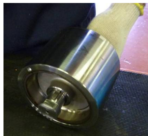
Fig. 42 Pull the impeller shaft (211) out of the inner magnet (855).
