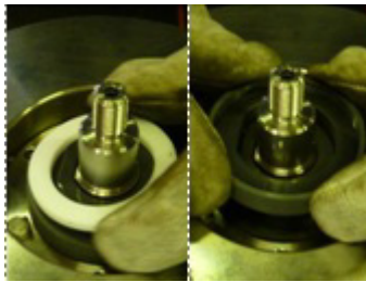
Fig. 39 Remove the compensation ring (504) and the front slewing bearing (510).
