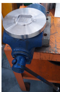
Fig. 35 Tighten the equipment (if available) in a bench vice and place the assembled bracket on top.
