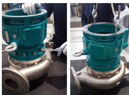
Fig. 32 Loosen the nuts (920) and separate the lantern (344) from the volute casing (102) using appropriate lifting systems.
