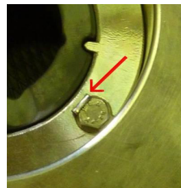
Fig. 54 For the "1st bracket" pumps: position the bushing locking flange (935) so that the anti-rotation tooth is aligned with the slot of the bearing bush (545). Tighten the screws (901), bend and lock the washers. Turn the support (350) upside down and repeat the same operations to assemble the other bearing bush (545).
