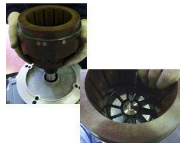
Fig. 58 Fit the outer magnet on the motor shaft (856). Screw in the screw (918) with relevant washer (555) using Loctite 243 threadlock to ensure they are tight.
