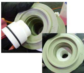
Fig. 53 Fit the bearing sleeves (529) into the impeller assembly (240).
