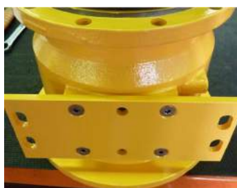
Fig. 44 Insert the antispark ring (516) in the relevant seat inside the lantern (344). Fig. 45 Fasten the spacer ring (892.1) to the lantern (344) by means of screws. Fig. 46 ONLY for SERIES 200: Screw in the screws to fasten the lantern (344) to the adapter flange (159) of the volute casing.
