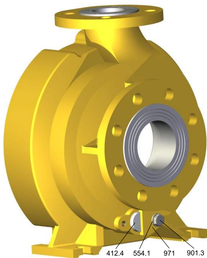
Fig. 26 UTN-BL special execution drawing with drained casing (see DIN code table on the previous page).
