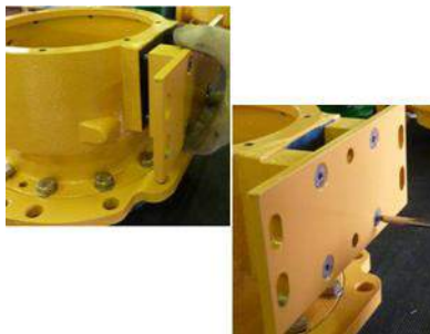
Fig. 48 ONLY for SERIES 200: Fasten everything to the lantern (344).
