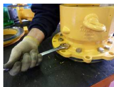
Fig. 41 ONLY for SERIES 200: Undo the screws to remove the lantern (344) from the adapter flange (159) of the volute casing.
