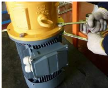
Fig. 28 Undo the screws to separate the lantern (344) from the motor.
