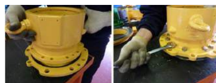
Fig. 44 Insert the antispark ring (516) in the relevant seat inside the lantern (344). Fig. 45 Fasten the spacer ring (892.1) to the lantern (344) by means of screws. Fig. 46 ONLY for SERIES 200: Screw in the screws to fasten the lantern (344) to the adapter flange (159) of the volute casing.
