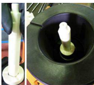
Fig. 51 Couple the static shaft (211) with the thrust bearing (510), which must have 3 splines toward the inner part of the shaft. Fit the shaft with bearing into the isolation shell (157) so that the 3 splines of the bearing are visible.
