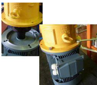
Fig. 59 Stand the pump on the motor with suitable lifting equipment. Screw the motor on the lantern (344) with the suitable screws.
