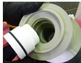
Fig. 35 Remove the bearing sleeves (529) with relevant locking O-ring (412.2) from the impeller assembly (240).
