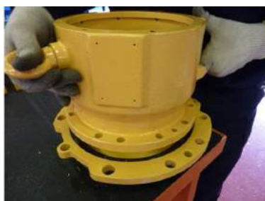
Fig. 42 ONLY for SERIES 200: Pull out the lantern (344) from the adapter flange (159) of the volute casing.
