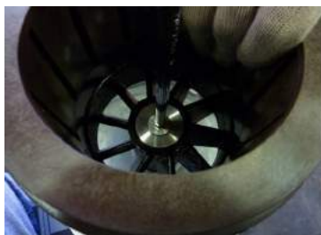
Fig. 30 Undo the screw (918) to remove the outer magnet (856) from the motor.
