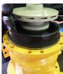
Fig. 54 Fit everything on the static shaft (211).
