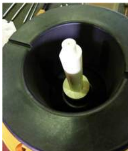
Fig. 36 Pull out the static shaft (211) and thrust bearing (510) from the isolation shell (157).
