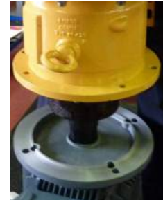
Fig. 29 Pull out the pump from the motor with the outer magnet (856) by means of suitable lifting equipment.
