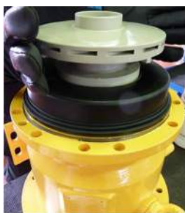
Fig. 34 Pull out the impeller assembly (240) from the shaft (211).
