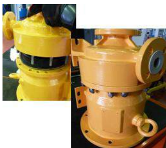
Fig. 57 Assemble the volute casing (102), including the already screwed in studs (902), on the lantern (344) by screwing the nuts and relevant washers. 243 threadlock to ensure they are tight.
