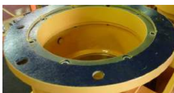
Fig. 40 Remove the motor flange (347) from the lantern (344) by undoing the relevant screws.
