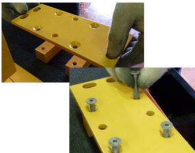
Fig. 47 ONLY for SERIES 200: Fasten the spacer rings (892.1-892.2) with the relevant screws.
