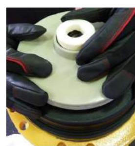
Fig. 55 Insert the thrust bearing (510) in the shaft (211) taking care to place the 3 splines toward the bearing sleeve (529).
