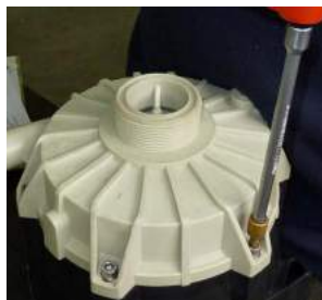
Fig. 50 Assemble the volute casing (102) on the lantern (344) tightening the relevant screws (914.1) with washers. Between the screws and washers, place the disc springs for ETFE or ETFE-CF casing and the grower springs for PP-GF casing.
