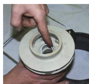
Fig. 46 Seat the bushing locking O-ring (412.2) into the impeller assembly (240).
