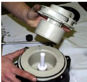
Fig. 48 Fit everything on the static shaft (211).
