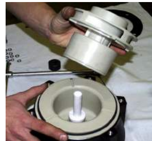
Fig. 27 Pull out the impeller assembly (240) from the shaft (211).
