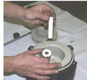
Fig. 30 Pull out the static shaft (211) and thrust bearing (510) from the isolation shell (157).
