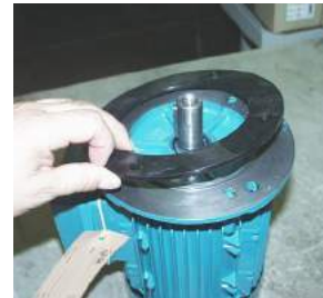
Fig. 36 Pull out the motor flange (347).
