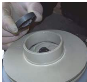
Fig. 49 Insert the thrust bearing (510) on the shaft (211).
