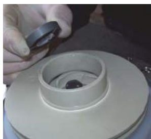
Fig. 26 Pull out the thrust bearing (510) from the shaft (211).
