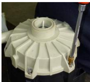
Fig. 25 Disassemble the volute casing (102) from the lantern (344) by unscrewing the relevant screws.
