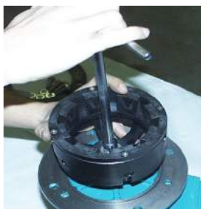
Fig. 38 Insert the motor flange (347) on the motor centring (for 100/112 motors having a B3-B14 construction, follow the relevant instructions indicated in the section "Disassembly of pump STN 30/40" in the chapter "Disassembly", in reverse order). Fig. 39 Fit the outer magnet on the motor shaft (856). Tighten the screw (918) with the relevant washer (555). Ensure the seal with threadlocker type Loctite 243. Screw in the grub screw (904). Fig. 40 Screw the motor on the lantern (344) with the suitable screws and washers.
