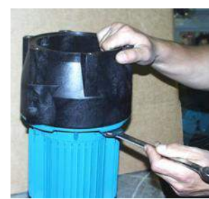
Fig. 33 Remove the motor with outer magnet (856) and the motor flange (347) from the lantern (344) by undoing the relevant screws.
