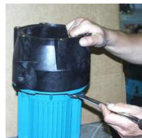
Fig. 38 Insert the motor flange (347) on the motor centring (for 100/112 motors having a B3-B14 construction, follow the relevant instructions indicated in the section "Disassembly of pump STN 30/40" in the chapter "Disassembly", in reverse order). Fig. 39 Fit the outer magnet on the motor shaft (856). Tighten the screw (918) with the relevant washer (555). Ensure the seal with threadlocker type Loctite 243. Screw in the grub screw (904). Fig. 40 Screw the motor on the lantern (344) with the suitable screws and washers.
