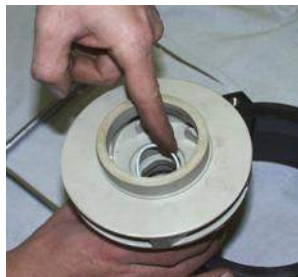
Fig. 29 Remove the bushing locking O-ring (412.2) from the impeller assembly (240).
