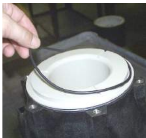
Fig. 31 Remove the O-ring (412.1) from the isolation shell (157).
