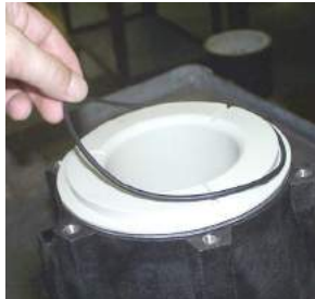
Fig. 42 Fit the O-ring (412.1) on the isolation shell (157).
