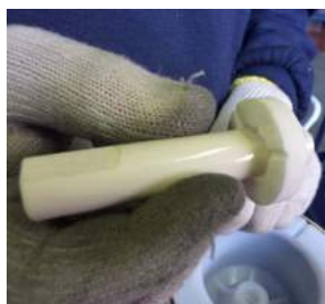
Fig. 44 Couple the static shaft (211) with the thrust bearing (510), which must have 3 splines toward the outmost part of the shaft.
