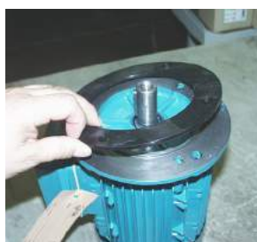
Fig. 38 Insert the motor flange (347) on the motor centring (for 100/112 motors having a B3-B14 construction, follow the relevant instructions indicated in the section "Disassembly of pump STN 30/40" in the chapter "Disassembly", in reverse order). Fig. 39 Fit the outer magnet on the motor shaft (856). Tighten the screw (918) with the relevant washer (555). Ensure the seal with threadlocker type Loctite 243. Screw in the grub screw (904). Fig. 40 Screw the motor on the lantern (344) with the suitable screws and washers.
