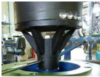
Fig. 34 Undo the grub screw (904) of the outer magnet (856).
