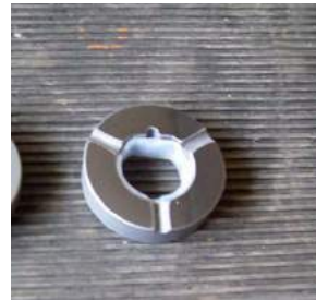
Fig. 43 Check that the bearing locking-setting ring in PFA plastic material (512) is inserted in the thrust bearing (510).
