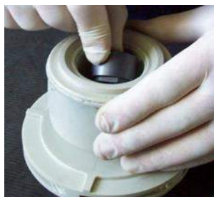
Fig. 28 Remove the bearing sleeves (529) from the impeller assembly (240).
