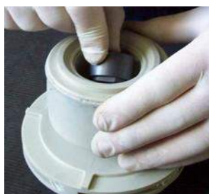
Fig. 47 Fit the bearing sleeves (529) into the impeller assembly (240).
