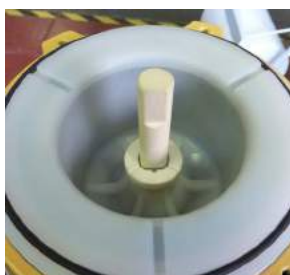
Fig. 45 Fit the shaft (211) with bearing (510) into the isolation shell (157) so that the 3 splines of the bearing are visible.
